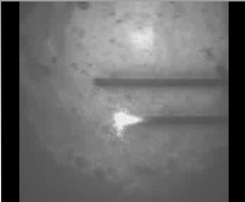
Laser ablation of alumina target (100 \mu\text{m} thickness)
