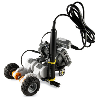
Figure 2 Our “magnet finder” using a side-mounted sensor holder
