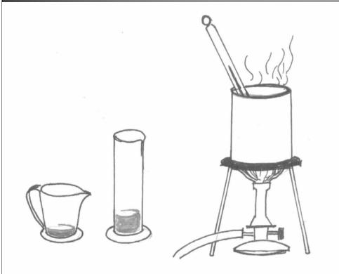
1. When it boils, add 200 ml cold water. 2. WATCH OUT: The temperature should NOT go above 110 °C!
