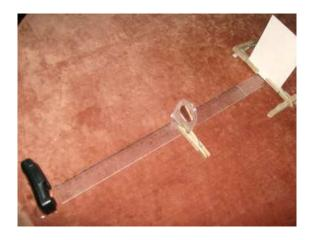
I noticed that as the object moves closer to the lens, the image moves away from the focal point. If the object is exactly at the focal point, there is no image formed at all. (The image distance is sometimes said to be "infinite.") In fact, if a point of light is placed at the lens focus, the rays are made parallel by the lens.
