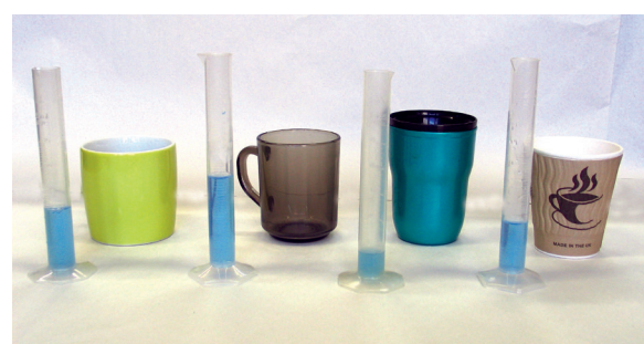
Testing insulation by melting ice
